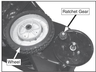
Figure 12. Wheel removed.
